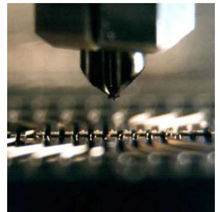
Fig 2 microgripper used as pull test tool
